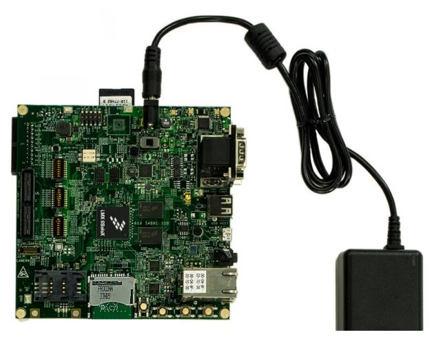
To power-on the board, connect the power supply to J1 and toggle SW1-PWRON switch.
